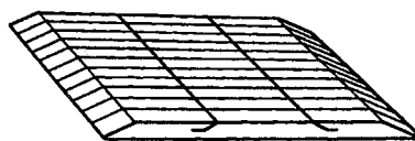
Figure 3.54 The Plate after Being Planed
